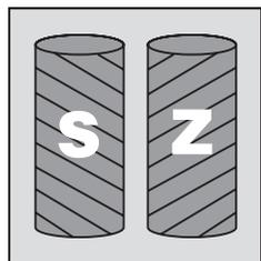
Timken ACHE (Air-Cooled Heat Exchanger) synchronous belts are manufactured using a special construction. Because the drive has a vertical shaft, the belt is built with "Z" twist cords only.
