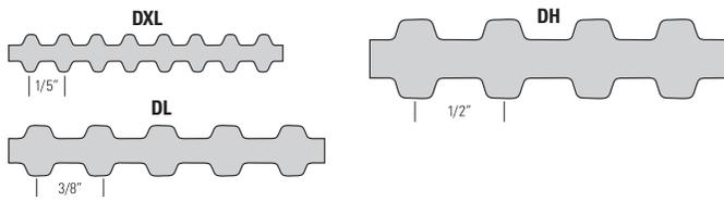
**Double-sided timing belt with a trapezoidal tooth profile provides synchronization and 100% load capacity from both sides of the belt.**
