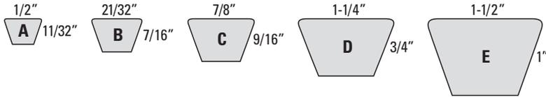
**Premium wrapped molded v-belt built to the highest standards in the industry. Ideal for classical drives with shock loads.**
