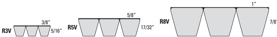
Super Power-Wedge Band (formerly Wedge-Band®) is the banded version of the hard-working Super Power-Wedge v-belt. The specially compounded wrapped construction is ideal for clutching operations. Super Power-Wedge Band is oil and heat resistant, static dissipating, and reduces the ability for a belt to turn over or jump off the drive.
