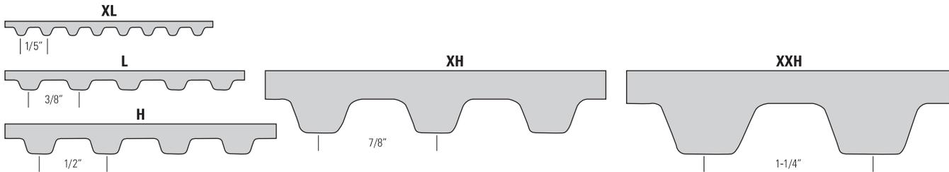
**The Synchro-Cog® Timing Belt has a trapezoidal tooth profile for applications where synchronization between the driving and driven units is required.**
