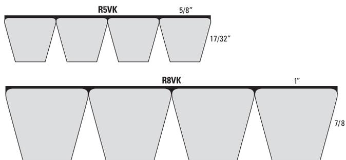
**Aramax® Super Power-Wedge® Bands are designed for extraordinary strength on the toughest drives.**
