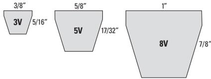
**Super Power-Wedge® v-belts enable the design of a more compact belt drive with controlled power transfer. The cover provides superior wear resistance and is ideal for heavy duty industrial drives with shock loads.**
