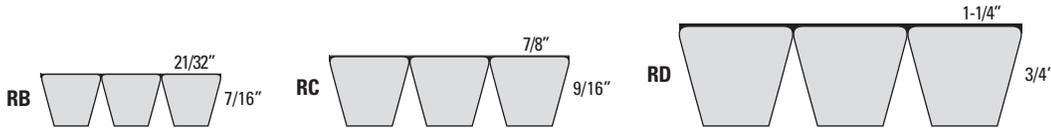
The banded version of our Super Blue Ribbon v-belt. Two or more Super Blue Ribbon v-belts are permanently joined together at the top with a reinforced tie-band. Ideally suited for pulsating or heavily shock loaded drives and drives with long center distances to minimize belt whip and rollover.
