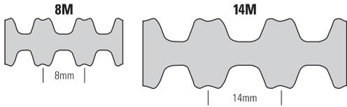
**Proven performance from both sides of the belt for greater flexibility and efficiency in your drive design.**
